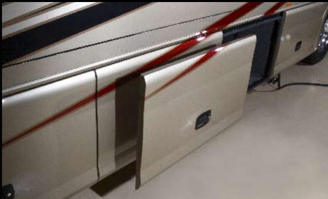
Horizontal parallel storage door for easy access to storage bay when slide room is extended.
